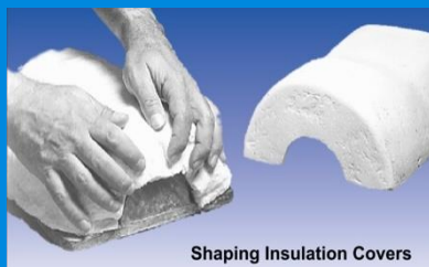
Shaping Insulation Covers
